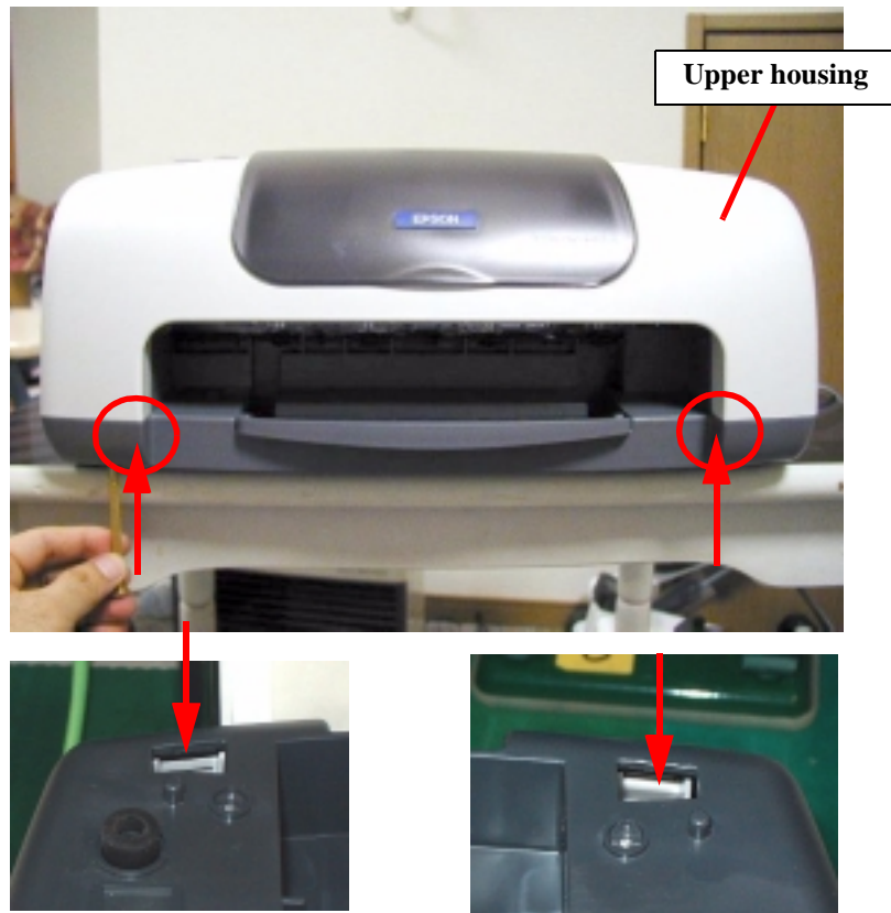
Figure 2-3. Removing the front hook
